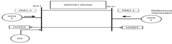
Fig 1: Configuration of the proposed hybrid distributed generation. (Import mode)
