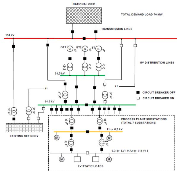
Fig.2. One line diagram of industrial facility electrical system showing generation, transmission and primary distribution systems
