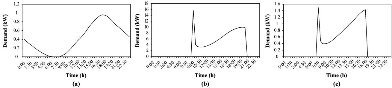
Fig. 4. Uncontrolled electrical load consumption curves. (a) Domestic air-conditioner. (b) Supermarket air-conditioner. (c) Office air-conditioner.
