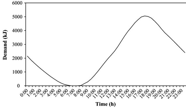
Fig. 1. Thermal load consumption curve for a domestic air-conditioner (flat).
