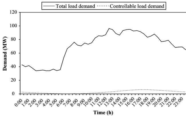
Fig. 5. Total and controllable load demand curves.
