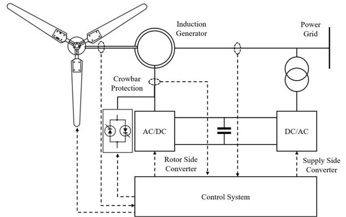
Fig. 1. Wind turbine DFIG configuration
