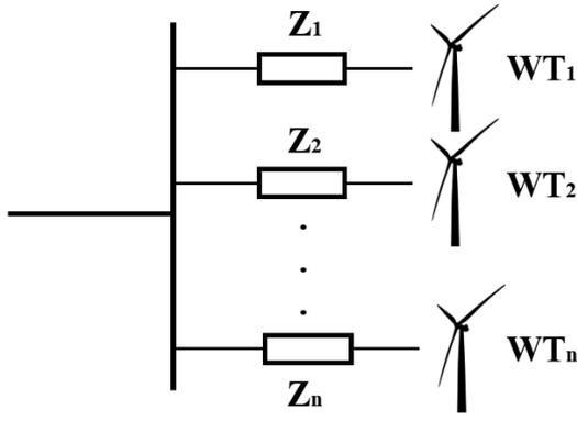
Fig. 2. Parallel connection of n wind turbines
