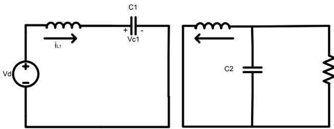
Fig. 1.c Cuk converter when switch is OFF
