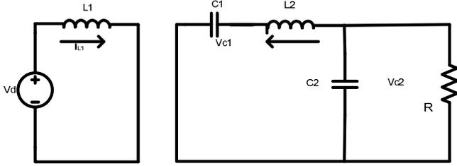
Fig. 1.b Cuk converter when switch is ON
