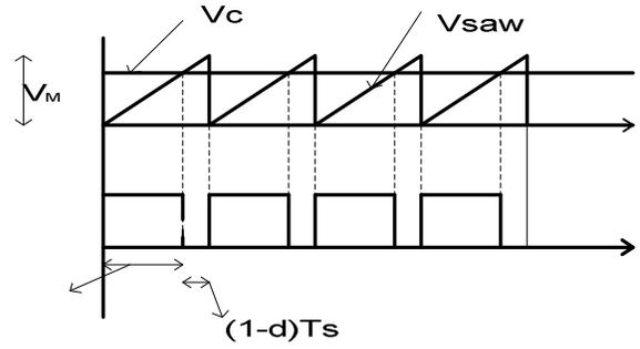
Fig.2.b waveform of PWM comparator
