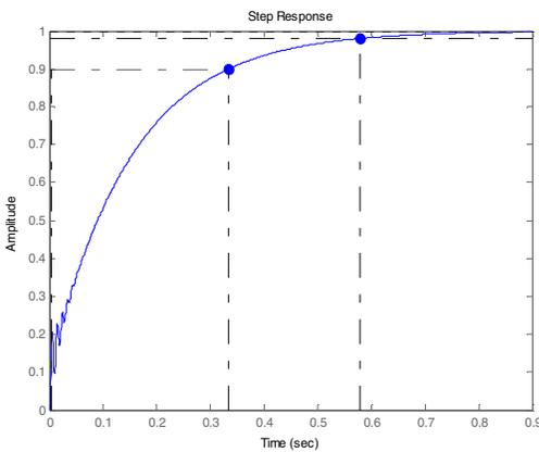
Fig.7 Step response of original system with compensator.
