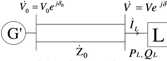
Fig. 3. An equivalent one-machine one-load decentralized system.
