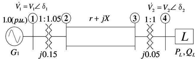
Fig. 7. The Japanese standard one-machine system model with load.
