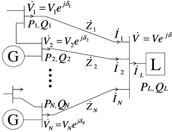
Fig. 2. Power flow at a load-bus.
