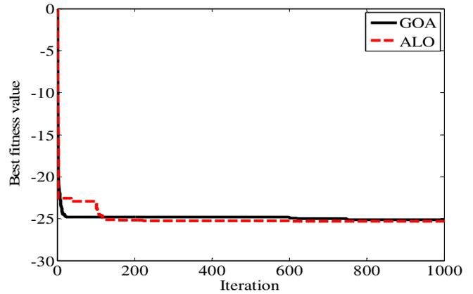
Figure 4: Convergence curve of ALO and GOA-optimized 10 elements LAA over 1000 iterations for the best run.
