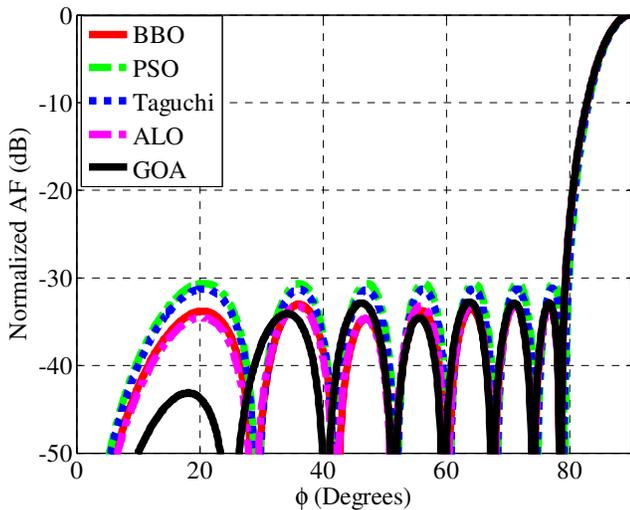
Figure 5: Radiation pattern of ALO and GOA-optimized 16-element LAA compared to other optimization techniques.
