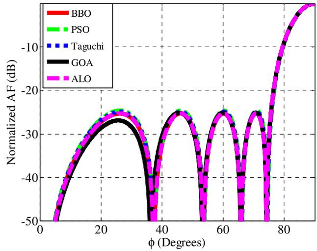
Figure 3: Radiation pattern of ALO and GOA-optimized 10-element LAA compared to other optimization techniques
