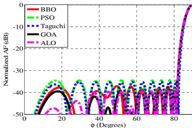
Figure 7: Radiation pattern of ALO and GOA-optimized 24-element LAA compared to other optimization techniques.
