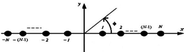
Figure 2: Geometry of the 2N element symmetric linear array.
