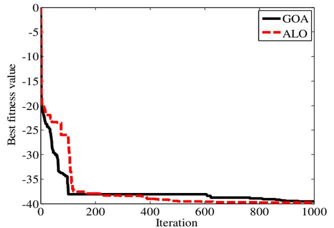
Figure 8: Convergence curve of ALO and GOA-optimized 24 elements LAA over 1000 iterations for the best run.
