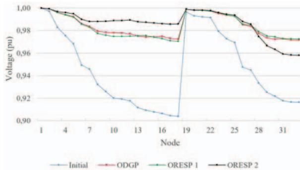
Figure 6 Voltage profile of 33-bus system
