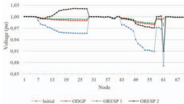
Figure 7 Voltage Profile of 69-bus system
