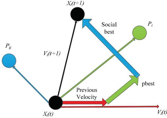
Figure 1 Vector diagram of a particle's movement
