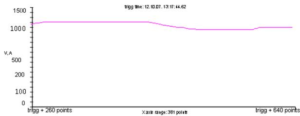
Fig 9(e): Measured dc output voltage waveforms of bridgeless PFC boost rectifier
