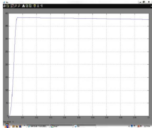
Fig 7(c): Measured dc output voltage waveforms of bridgeless PFC boost rectifier operating at 85-Vrms line voltages.  $V_{out} = 384V_{dc}$
