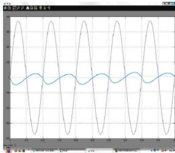
Fig 7(d) : Measured line voltage and line current waveforms of bridgeless PFC boost rectifier operating at 264-Vrms line voltage.
