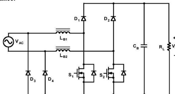
Fig 6: Bridgeless PFC rectifier with two DC/DC Boost Circuits
