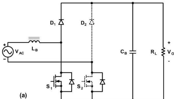
Fig. 5(a) Positive Half cycle of Basic bridgeless PFC boost rectifier
