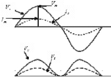
Fig 1b: Waveforms of related voltages and current
