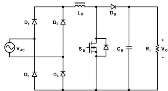
Fig 4: Conventional PFC Boost Rectifier
