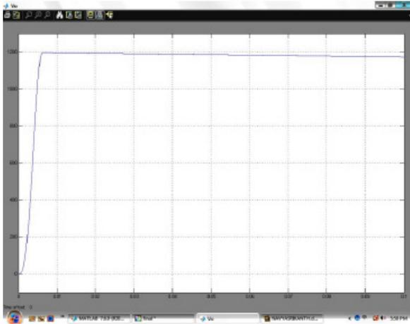
Fig 7(e): Measured dc output voltage waveforms of bridgeless PFC boost rectifier operating at 264-Vrms line voltages.  $V_{out}=1200$  Vdc
