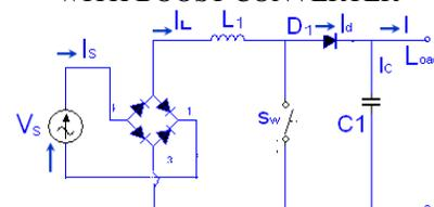
Fig 1a: Rectifier with Boost Converter
