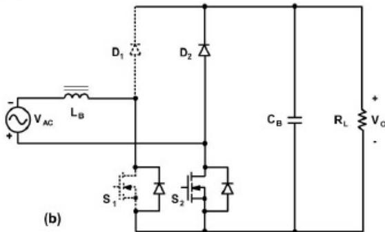
Fig 5(b): Negative Half cycle of Basic bridgeless PFC boost rectifier
