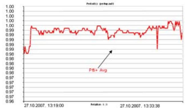
Fig 9(C): Power factor with PFC
