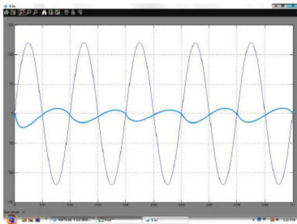
Fig 7(b) : Measured line voltage and line current waveforms of bridgeless PFC boost rectifier operating at 85-Vrms line voltage
