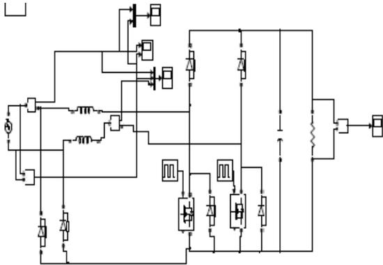
Fig 7(a): Bridgeless PFC rectifier with two DC/DC Boost Circuits
