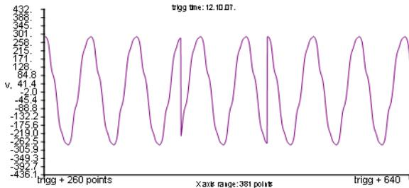
Fig 9(d) : Measured line voltage and line current waveforms of bridgeless PFC boost rectifier
