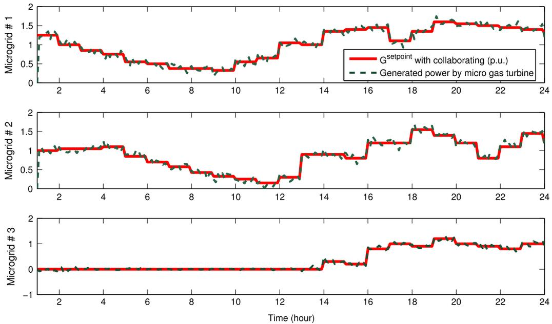
Fig. 6. The generated power from the micro gas turbine in the three microgrids versus the residual demand.
