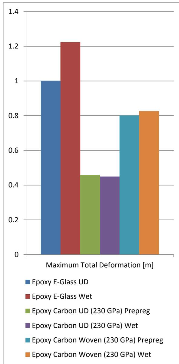
**Figure 17:** Tip maximum total deformation in meters
