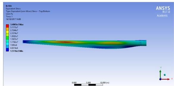
**Figure 8:** Equivalent (von-Mises) stress distribution along the blade for Material 3
