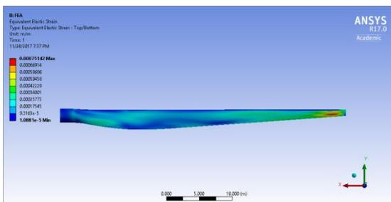
**Figure 23:** von-Mises Strain distribution along the blade for Material 4
