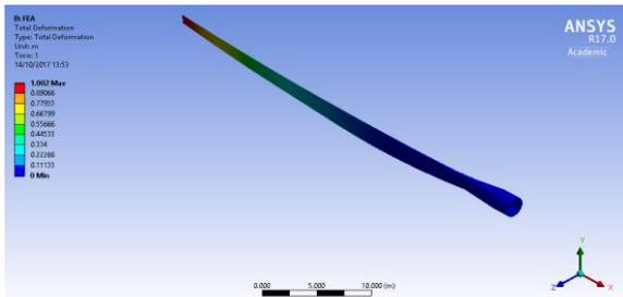
**Figure 3:** Deformation distribution along the blade for Material 1
