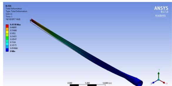
**Figure 7:** Deformation distribution along the blade for Material 3
