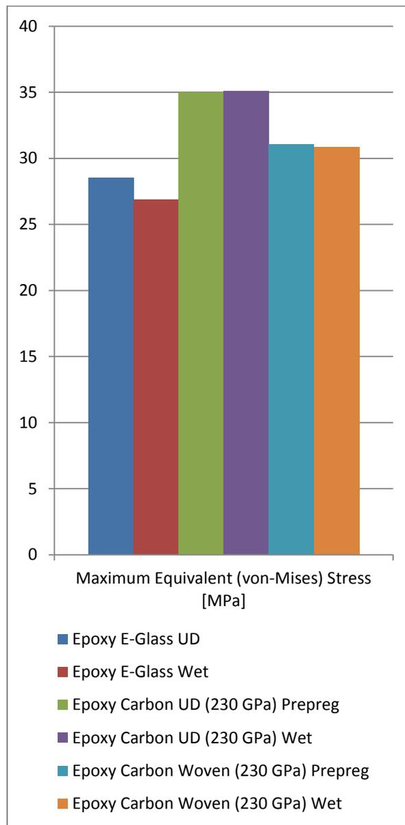
**Figure 18:** Maximum equivalent (von-Mises) stresses in MPa
