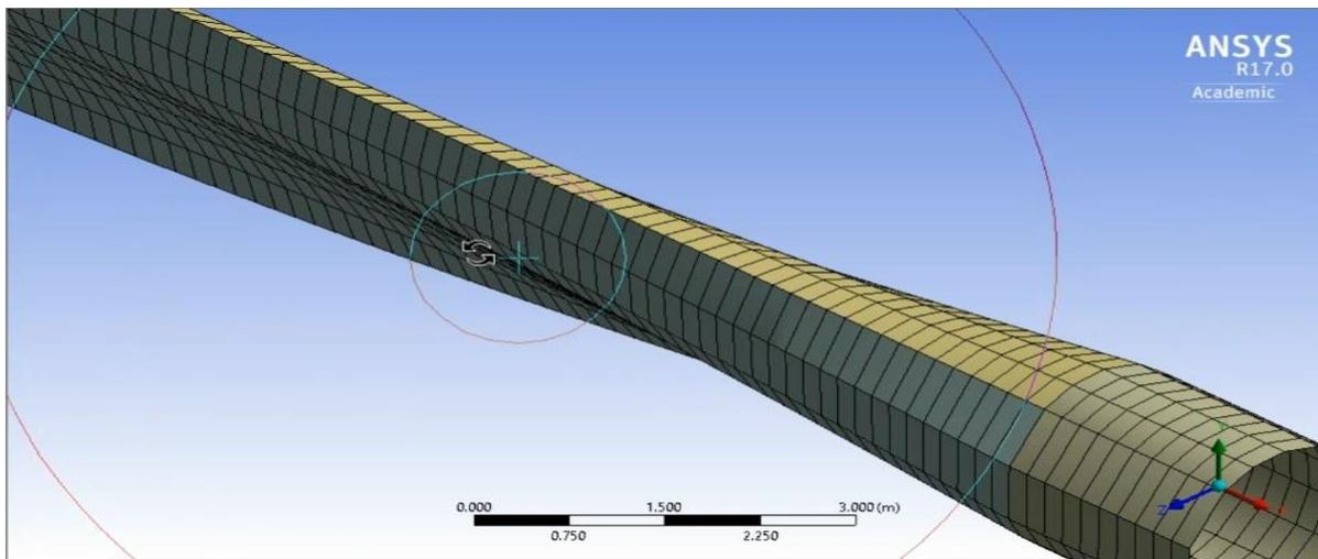
**Figure 2:** The Finite Element Method mesh generated by ANSYS
