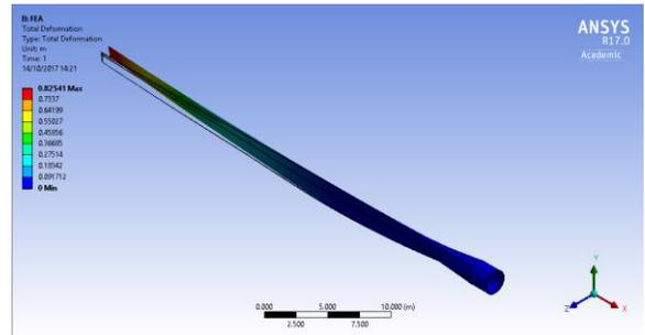
**Figure 13:** Deformation distribution along the blade for Material 6
