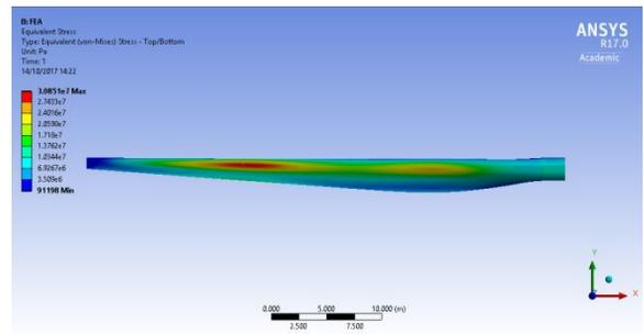
**Figure 14:** Equivalent (von-Mises) stress distribution along the blade for Material 6
