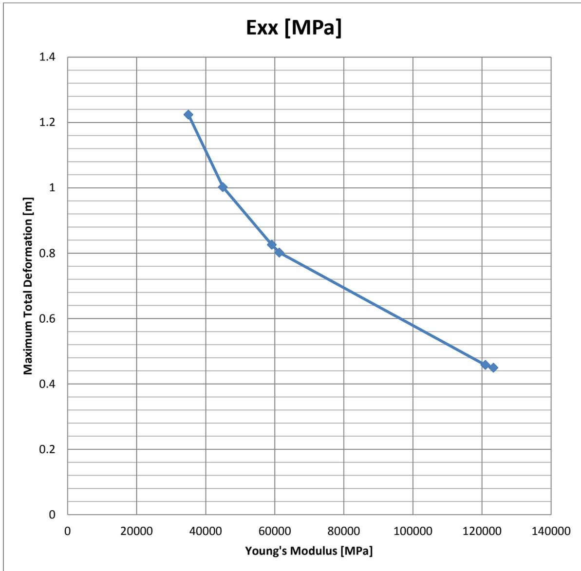
**Figure 16:** Tip total deformation of the wind turbine blade decreasing with the increase in Young's modulus in the x direction. Each point on the plot represents a material.
