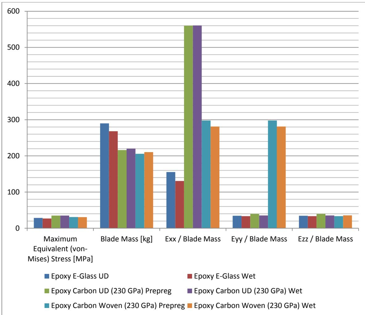
**Figure 20:** Young's modulus per unit mass of the blade for the x, y, and z directions
