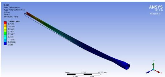
**Figure 11:** Deformation distribution along the blade for Material 5
