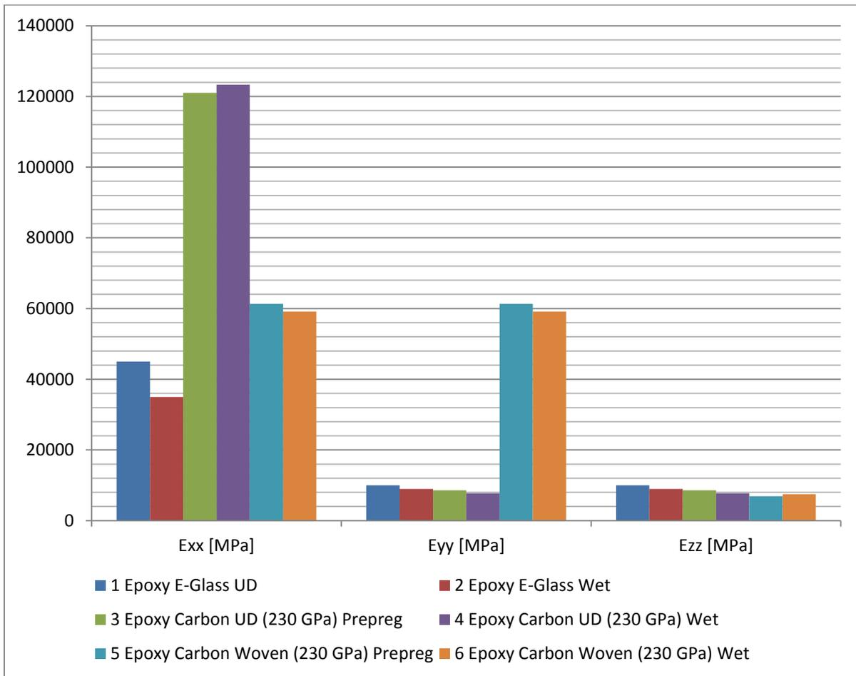
**Figure 15:** Young's modulus in the x, y, and z directions for the simulated materials in the paper represented graphically
