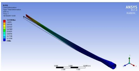
**Figure 5:** Deformation distribution along the blade for Material 2
