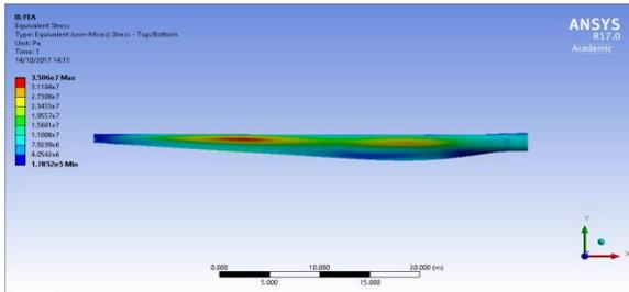
**Figure 10:** Equivalent (von-Mises) stress distribution along the blade for Material 4
