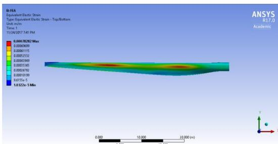
**Figure 21:** von-Mises Strain distribution along the blade for Material 1
