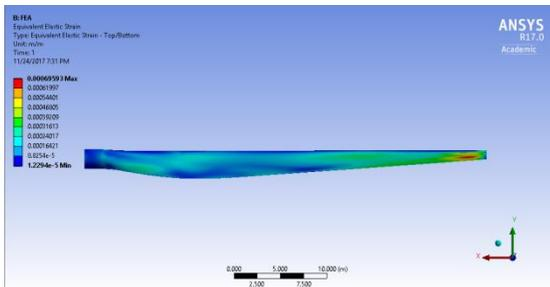
**Figure 22:** von-Mises Strain distribution along the blade for Material 3
