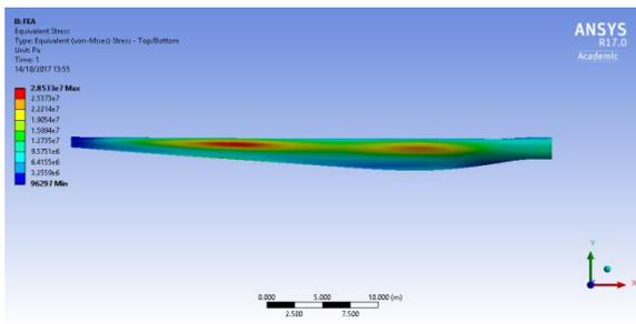
**Figure 4:** Equivalent (von-Mises) stress distribution along the blade for Material 1
