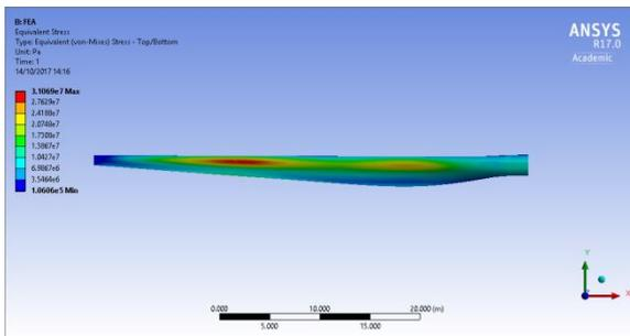
**Figure 12:** Equivalent (von-Mises) stress distribution along the blade for Material 5
