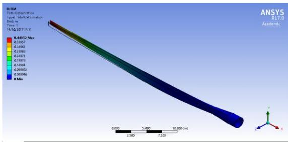
**Figure 9:** Deformation distribution along the blade for Material 4
