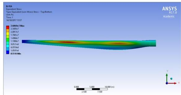
**Figure 6:** Equivalent (von-Mises) stress distribution along the blade for Material 2
