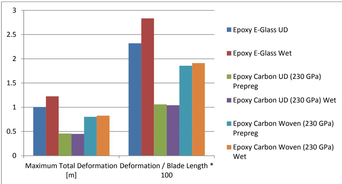
**Figure 19:** Tip maximum total deformation in meters and in percentage of the blade length results obtained from the ANSYS computer simulation for each of the materials simulated
