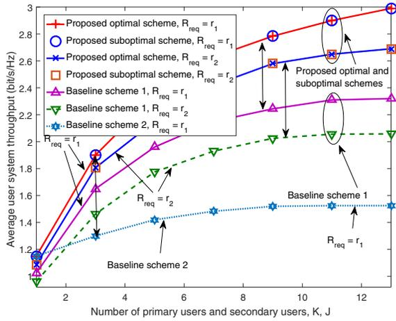
Fig. 4. Average user system throughput (bit/s/Hz) versus the number of primary and secondary users,  $K, J$ , for different resource allocation schemes. The double-sided arrows indicate the performance gains of the proposed optimal scheme compared to the baseline schemes.
