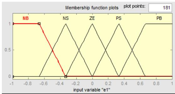
Fig. 3(a): Membership function of Error signal
