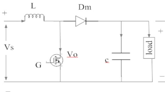
Fig.1 - DC-DC Boost Converter
