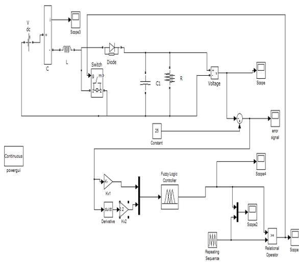
Fig.4 Simulink Model for Boost Converter with FLC Controller
