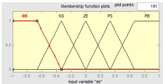
Fig. 3 (b) Member function of Derivative signal
