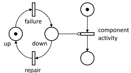
Fig. 7. Failure model of a system component.
