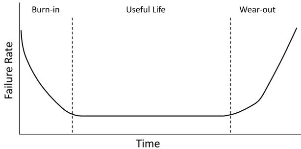
Fig. 2. Bathtub curve for hardware reliability [12].
