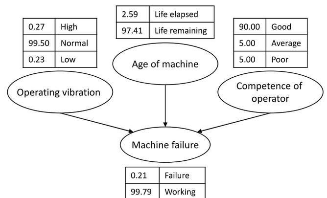
Fig. 8. Bayesian network for a machine failure.
