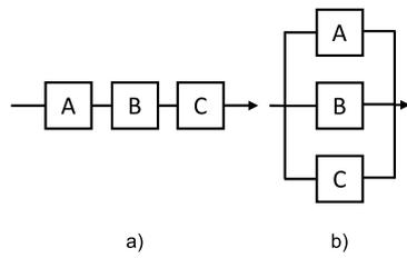
Fig. 5. RBD with system in sequential (a) and parallel (b) configuration.
