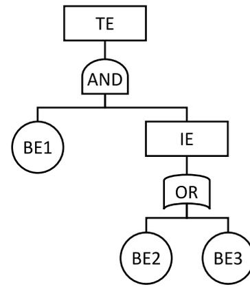
Fig. 6. Fault tree with top (TE), intermediate (IE) and basic events (BE).
