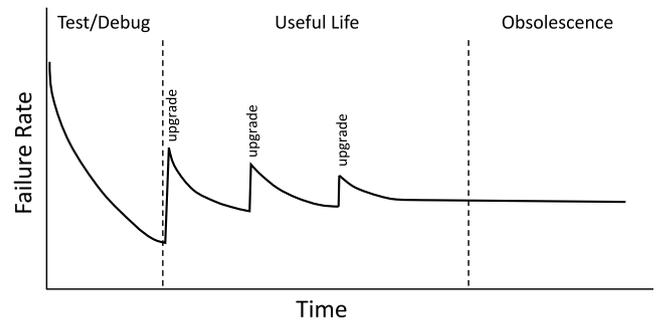
Fig. 3. Revised bathtub curve for software reliability [12].
